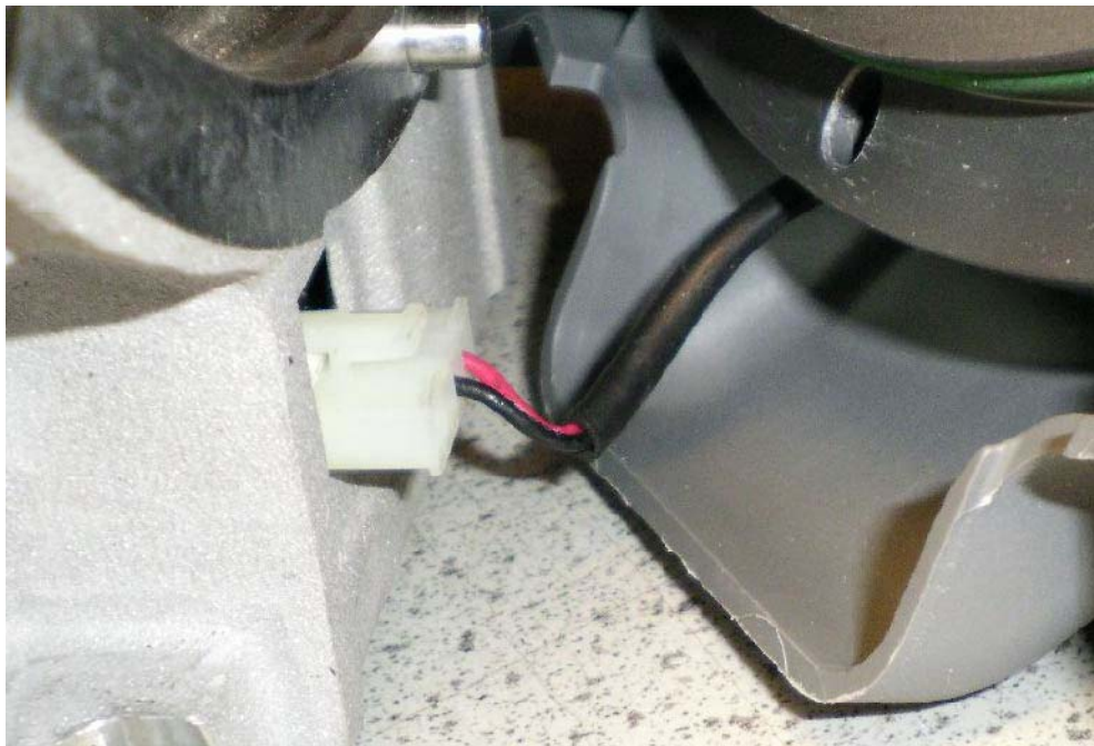
Figure 3 - Motor fan lead connector
