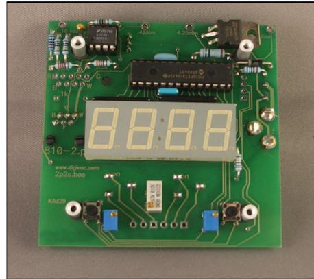
The various test points are at the top of the board and are identified with writing. For user recalibrations, it is only necessary to adjust the zero pot. It can be reached through a hole in the front panel, so disassembly is not necessary.
