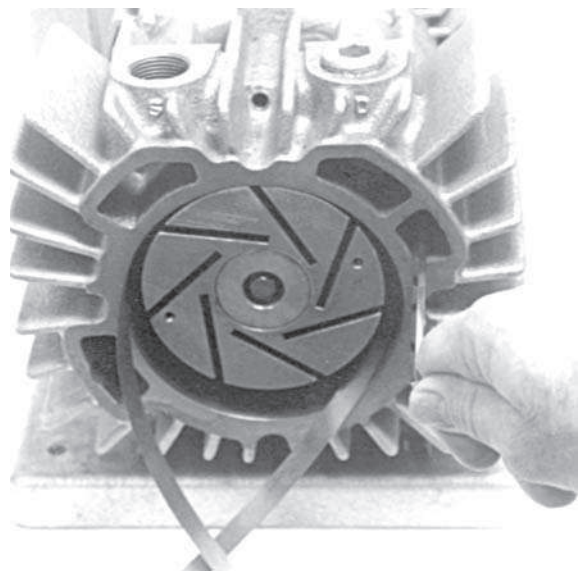
Fig. 16 - Setting the Radial Clearance
