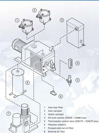
Industrial oil sealed pumps are used in a wide variety of applications and produce reliable vacuum for many processes. To optimize the installation and to prolong pump life, Edwards offers a range of accessories for our large oil-sealed pumps. Our pumps and accessories are designed to ensure that accessories are easy to install.
