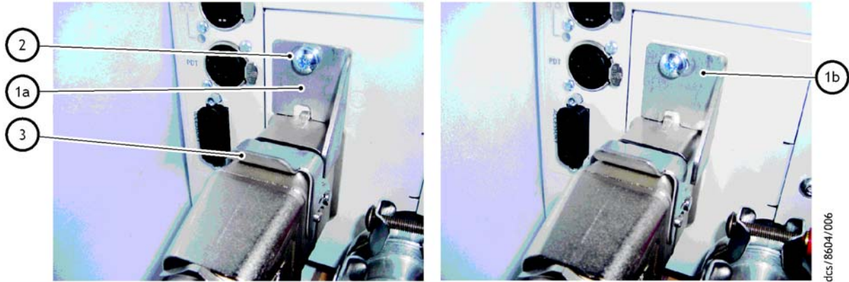
Figure 6 - Electrical connector locking mechanism
