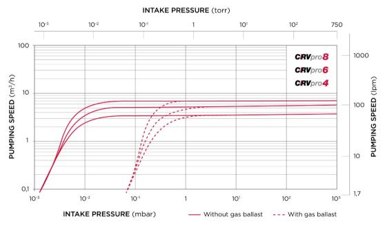
Fig. 6 Pumping Speed / Intake Pressure - Diagram CRVpro 4, 6, 8
