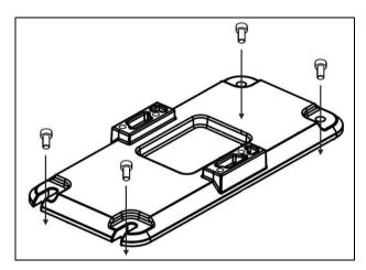
Fig. 8 Pump mounting
