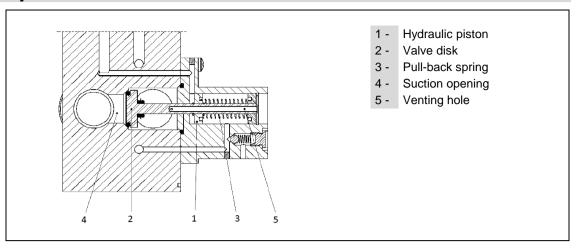
Fig. 4 Suction port valve (HV-valve)
