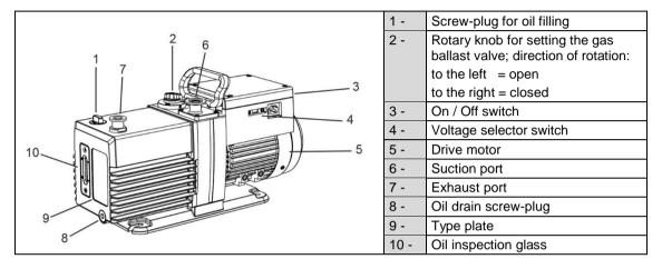
Fig. 1 Rotary vane vacuum pump (CRVpro 4, 6, 8)
