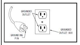
Fig. 9 Grounding plug illustration
