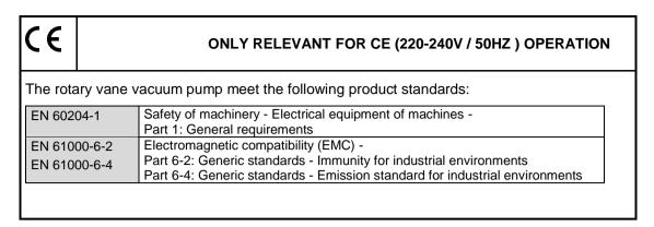
Observe the standards and regulations applying in your country when you use the rotary vane vacuum pump.
