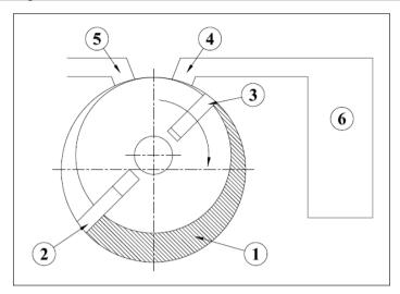
Fig. 2 Rotary vane vacuum pump Principle
